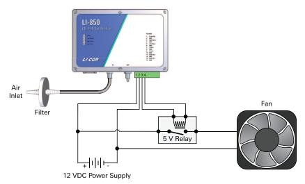
Figure 2-4. In this example, the high alarm is used to activate a relay, which turns on a fan.
