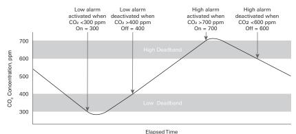
Figure 2-2. An alarm is triggered when a concentration is outside of a threshold. For example, the low alarm is activated if the concentration drops below 300 ppm and is deactivated when the concentration rises above 400 ppm. The high alarm is activated if the  $CO_2$  concentration exceeds 700 ppm. The alarm remains activated until the concentration drops below 600 ppm.
