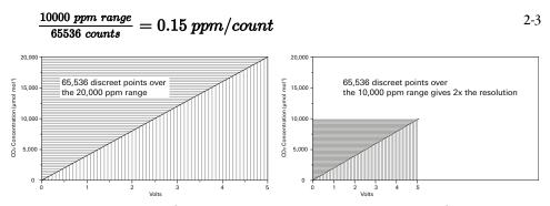
Figure 2-1. The resolution of the analog outputs depends upon the range. If the DACs are configured to output data over the full 0 to 20,000 ppm range, the data output over the DACs will have lower resolution (left). If the DACs are configured to output data over a narrower range (for example, 0 to 10,000 ppm as shown on the right), the data output over the DACs will have higher resolution.
